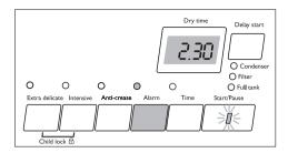
To deselect the function press the *Alarm* button again. The LED above is off.
